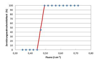
Picture-Caption: Measured laser damage threshold of a 45° mirror for 1030nm with 210fs pulses
