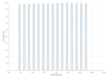
Theory curve of a multi-bandpass w/15 transmission channels; individual channels are separated from each other by OD6 block bands. Measurement curves of concrete customer projects are subject to confidentiality.
