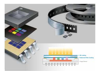
Sensor Package for Ambient Light Sensing
