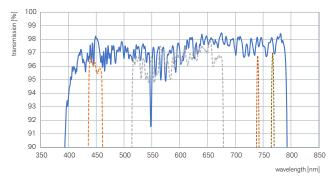
Fig. 4: High transmission level >97% for different filter configurations
