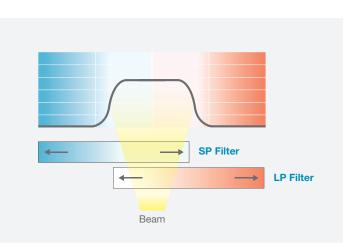
Fig. 6: LVF based on the combination of LP-filter and SP-filter
