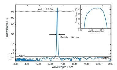
Fig. 5: Spectral range with absolut blocking >OD4 and average blocking >OD5
