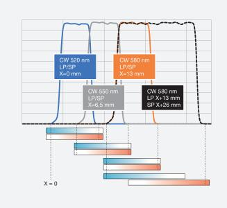
Fig. 7: Bandpass filter adjustment for tuning of different filter characteristics
