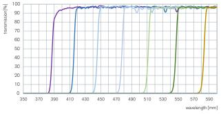
Fig. 3: Individual edge positions in the spectral range and their transmission value
